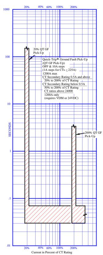
Quick-Trip® Ground Fault Time Current Curve
